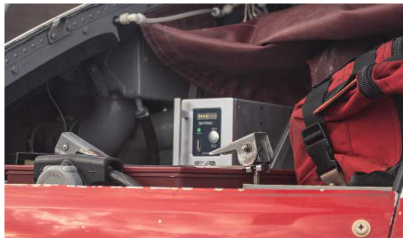
The ISAT-200A powered on and onboard Alpine's Bell 212 HP Helicopter.
