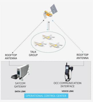
Figure 6. Encrypted Satellite Push-to-Talk through LEO (Iridium).
