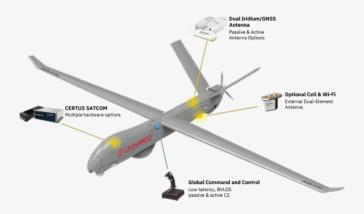
Figure 8. DLS-100 and IMS-350 UAV Satcom configurations.
