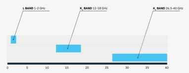
Figure 3. Satcom spectrum bands by GHz profile.
