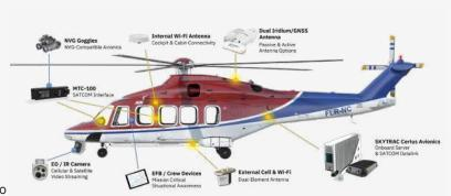
Figure 4. Critical components relying on Satcom on a modern SAR helicopter.
