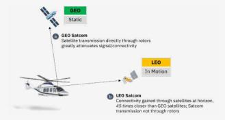
Figure 2. LEO versus GEO satellite connectivity comparison.
