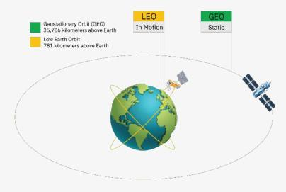
Figure 1. LEO versus GEO motion and distance from Earth (not to scale).
