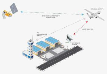
Figure 7. Satcom Beyond Line of Sight Communications with UAV.
